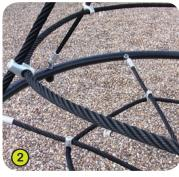
**2- The Polyfix rope**,  $\varnothing$  16 mm, is made up of six,  $\varnothing$  0.8 mm, galvanised steel cables. The rope is covered with polypropylene.
