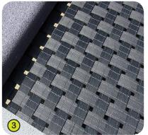
**3- The trampoline surface** is made up of a series of straps, reinforced with steel cables; the straps are joined to the frame by steel springs, each 185mm long and 20mm in diameter.
