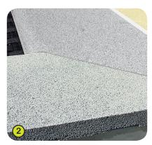
**2- The tiles** are made from 30mm thick Euroflex rubber.
