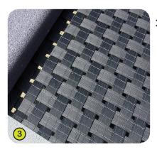
**3- The trampoline surface** is made up of a series of straps, reinforced with steel cables; the straps are joined to the frame by steel springs, each 185mm long and 20mm in diameter.
