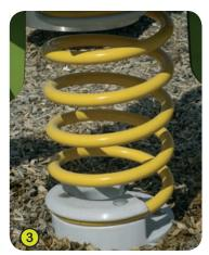
**3- The spring** is made from Grade 35SCD6 steel, shot blasted, stress relieved, zinc coated and finished with two coats of epoxy polyester powder.
