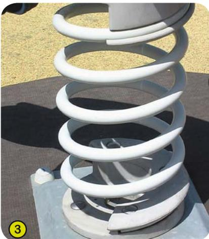
3- **The springs** are made from Grade 35SCD6 steel, shot blasted, stress relieved, zinc coated and finished with two coats of epoxy polyester powder. Proludic have patented an exceptionally strong and secure polyamide fixing for the spring, ensuring a long product life.
