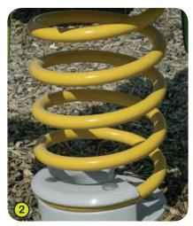
2- The spring is made from Grade 35SCD6 steel, shot blasted, stress relieved, zinc coated and finished with two coats of epoxy polyester powder. Proludic have patented an exceptionally strong and secure polyamide fixing for the spring, ensuring a long product life.
