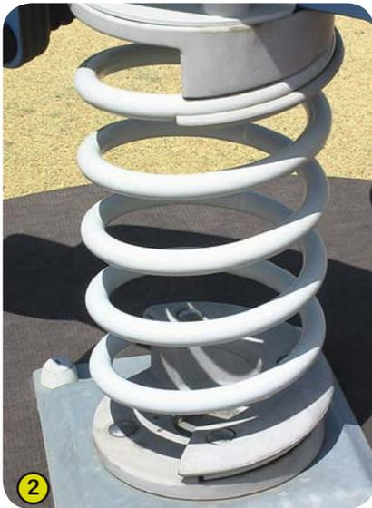
2- **The springs are** made from Grade 35SCD6 steel, shot blasted, stress relieved, zinc coated and finished with two coats of epoxy polyester powder. Proludic have patented an exceptionally strong and secure polyamide fixing for the spring, ensuring a long product life.
