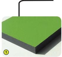
1- The coloured panels are made with a compact material 13mm thick. It is made up of 70% of softwood fibres and 30% of thermosetting resin, and it stands up to weathering very well (sun, rain, damp, etc.). The coloured surfaces are treated with products based on coloured acrylic polyurethane resins; this enables them to stand up well to UV radiation and resist damage.
