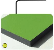
1- The coloured panels are made with a compact material 13mm thick. It is made up of 70% of softwood fibres and 30% of thermosetting resin, and it stands up to weathering very well (sun, rain, damp, etc.). The coloured surfaces are treated with products based on coloured acrylic polyurethane resins; this enables them to stand up well to UV radiation and resist damage.
