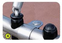
4- The platform is made from a textured and non-slip compact material (HPL), 19mm thick. The surface is circled with a 40mm diameter stainless steel tube.
