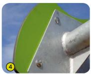
**4- The coloured panels** are manufactured from 13mm composite compact made up of softwood fibre (70%) and phenolic binder (30%). The material offers excellent resistance in all weather conditions (sun, rain, humidity...).
