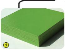
1- The lacquered panels are made from very high quality plywood 22mm thick. Made of alternate layers of thin birch, which offers longevity and an exceptional mechanical strangth. The colours are applied by electrostatic spraying of two-component polyurethane lacquer that is free of heavy metals, to ensure high levels of resistance to potentially aggressive chemicals such as anti-graffiti cleaning products.
