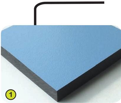
1- **The coloured panels** are made with a compact material 13mm thick. It is made up of 70% of softwood fibres and 30% of thermosetting resin, and it stands up to weathering very well (sun, rain, damp, etc.). The coloured surfaces are treated with products based on coloured acrylic polyurethane resins; this enables them to stand up well to UV radiation and resist damage.
