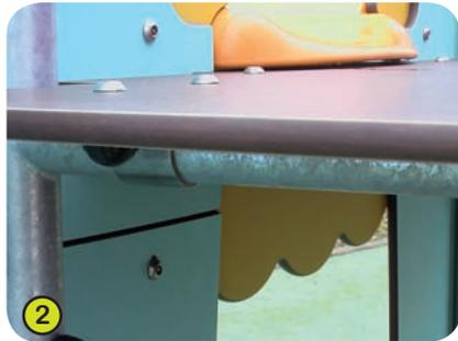
2- **The platforms** are made from a 12.5mm thick, textured, non-slip compact material (HPL). Further reinforcement is provided by galvanised steel supports.
