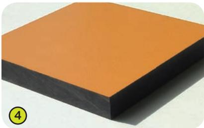
4- The coloured panel is made from a 13mm thick compact material (HPL).
