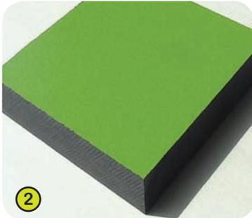
2- **The coloured panels** are made with a compact material 13mm thick. It is made up of 70% of softwood fibres and 30% of thermosetting resin, and it stands up to weathering very well (sun, rain, damp, etc.). The coloured surfaces are treated with products based on coloured acrylic polyurethane resins; this enables them to stand up well to UV radiation and resist damage.
