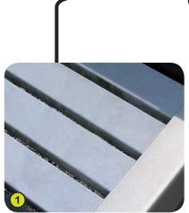
**1- The seat** is a combination of painted steel, 50x25x2.5mm, and pultruded polyester slats (compact polyester / fibre glass) 58x25x3mm, RAL 7004.
