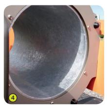
4- The tunnel is made of galvanised steel.
