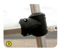
3- Injection moulded polyamide fixings connect the posts with the platforms and the various play features. They are non-toxic, flame shock and U.V. resistant. The thickness of the polyamide makes the equipement both strong and vandal resistant.
