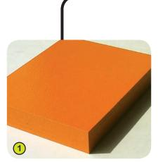
1- The lacquered panels are made from very high quality plywood 21mm thick. Made of alternate layers of thin birch, which offers longevity and an exceptional mechanical strangth. The colours are applied by electrostatic spraying of two-component polyurethane lacquer that is free of heavy metals, to ensure high levels of resistance to potentially aggressive chemicals such as anti-graffiti cleaning products.
