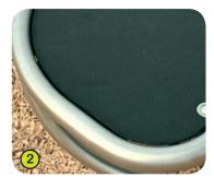
**2- The "Durax" platform floors** are machined from 22mm plywood panels made up of fine layers of birch. The surface is coated with a non-slip thermoplastic polyolefin film, and circled with a 40mm diameter stainless steel tube.
