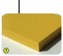
1- The lacquered panels are made from very high quality plywood 21mm thick, made of alternate layers of thin birch, which offers longevity and an exceptional mechanical strangth. The colours are applied by electrostatic spraying of two-component polyurethane lacquer that is free of heavy metals, to ensure high levels of resistance to potentially aggressive chemicals such as anti-graffiti cleaning products.
