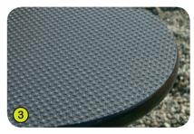
**3- The large beams** are 22mm thick panels made up of alternating layers of birch and pine. The surface is coated with a film of anti-slip phenolic resin.
