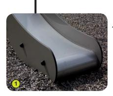
1- The sliding surface is made of stainless steel 2mm thick, which are shaped, bent and rolled from one piece.
