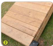
**2- The boards** are made of planks in solid pine wood, 145x46mm.
