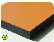
**4- The information panels** are made with a compact material 13mm thick. It is made up of 70% of softwood fibres and 30% of thermosetting resin, and it stands up to weathering very well (sun, rain, damp, etc.). The coloured surfaces are treated with products based on coloured acrylic polyurethane resins; this enables them to stand up well to UV radiation and resist damage.
