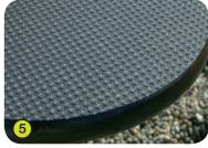
5- The panels (JPS16J and JPS16S) are 22mm thick panels made up of alternating layers of birch and pine. The surface is coated with a film of anti-slip phenolic resin.
