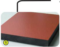
1- The coloured panels are made with a compact material 13mm thick. It is made up of 70% of softwood fibres and 30% of thermosetting resin, and it stands up to weathering very well (sun, rain, damp, etc.). The coloured surfaces are treated with products based on coloured acrylic polyurethane resins; this enables them to stand up well to UV radiation and resist damage.
