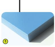
1- The lacquered panels are made from very high quality plywood 21mm thick, made of alternate layers of thin birch, which offers longevity and an exceptional mechanical strangth. The colours are applied by electrostatic spraying of two-component polyurethane lacquer that is free of heavy metals, to ensure high levels of resistance to potentially aggressive chemicals such as anti-graffiti cleaning products.
