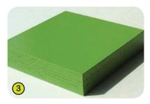
3- The lacquered panels are made from very high quality plywood 21mm thick, made of alternate layers of thin birch, which offers longevity and an exceptional mechanical strangth. The colours are applied by electrostatic spraying of two-component polyurethane lacquer that is free of heavy metals, to ensure high levels of resistance to potentially aggressive chemicals such as anti-graffiti cleaning products.
